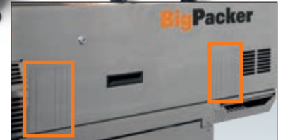
Preliminary cuts for installation of a continuous inkjet printer
